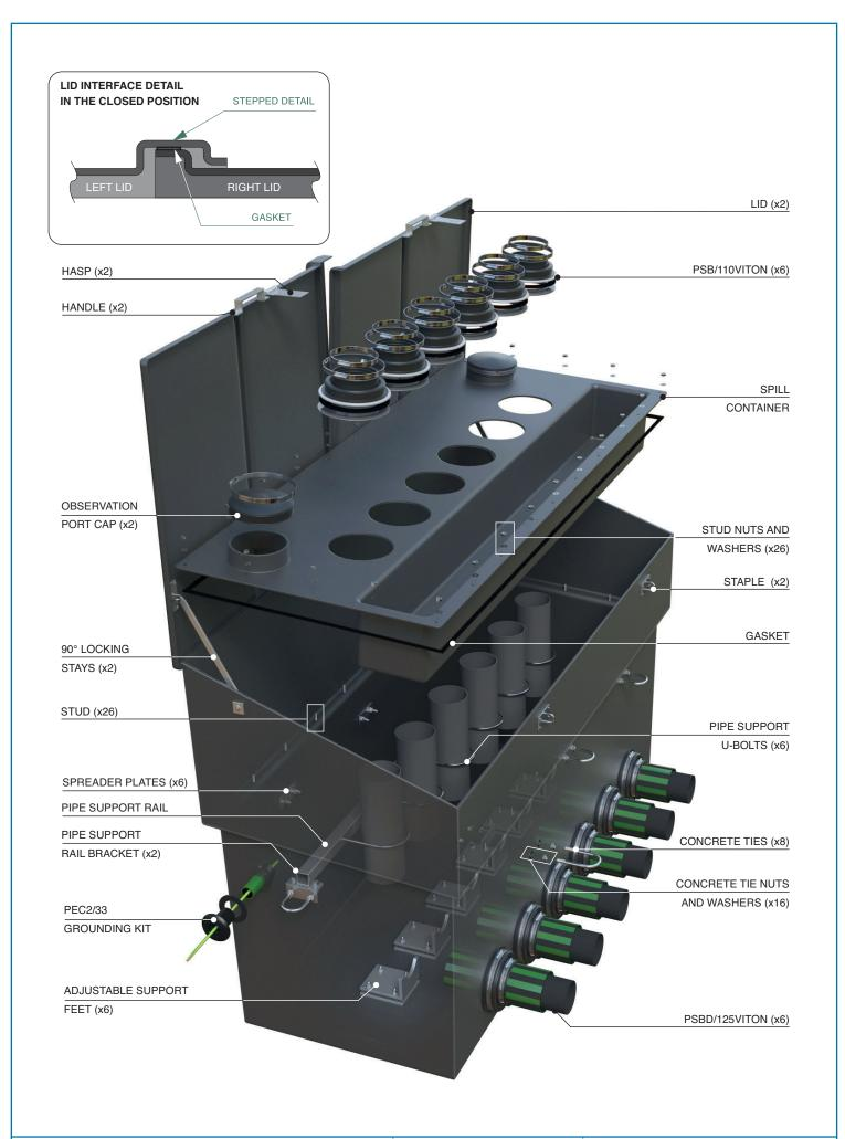
1737 x 686 x 1257mm deep GRP above ground fill sump with hinged double door to fit up to 6 fill lines. System includes internal spill tray, pipework support rail and concrete tie fixings.
