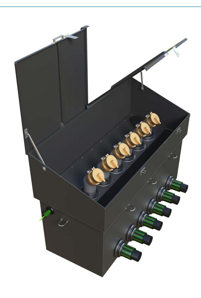
1737 x 686 x 1257mm deep GRP above ground fill sump with hinged double door to fit up to 6 fill lines. System includes internal spill tray, pipework support rail and concrete tie fixings.
