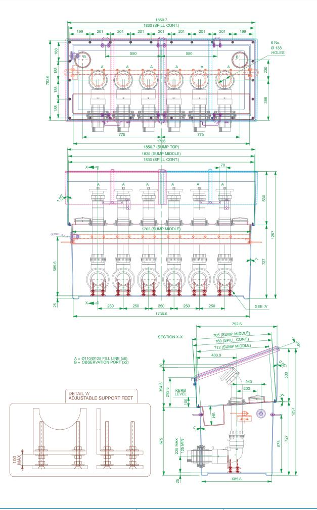
1737 x 686 x 1257mm deep GRP above ground fill sump with hinged double door to fit up to 6 fill lines. System includes internal spill tray, pipework support rail and concrete tie fixings.
