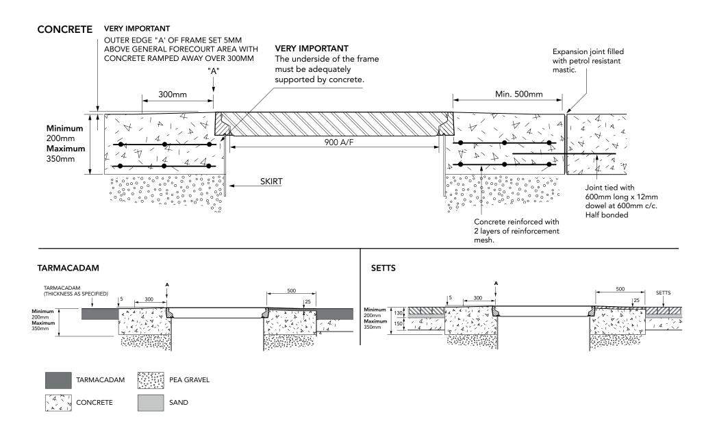
900mm diameter flat sealed composite cover with a composite frame.
