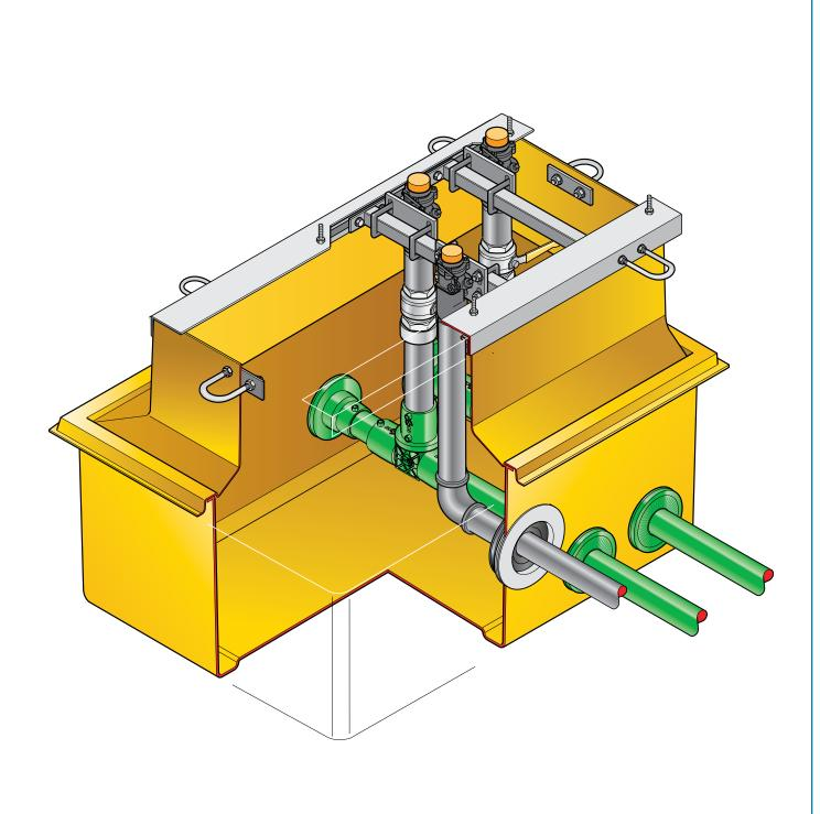
1100mm x 800mm GRP solid base sump and corbel to fit Tokheim Quantium Q510 dispenser model. Includes metalwork. KPS pipework.
