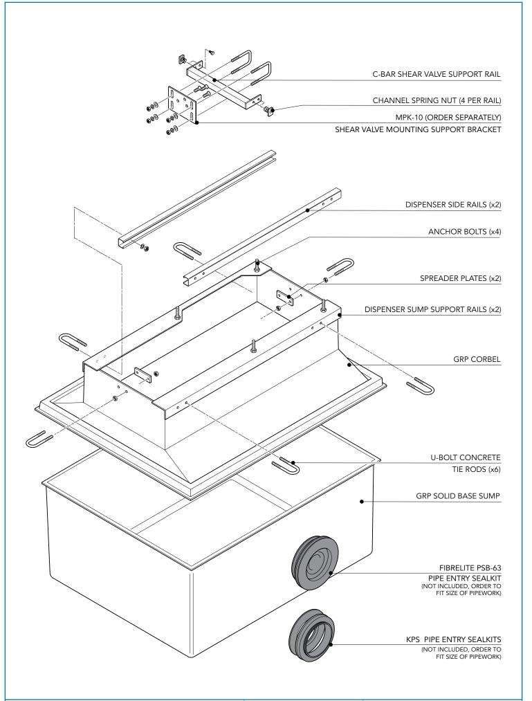
1100mm x 800mm GRP solid base sump and corbel to fit Tokheim Quantium Q510 dispenser model. Includes metalwork. KPS pipework.
