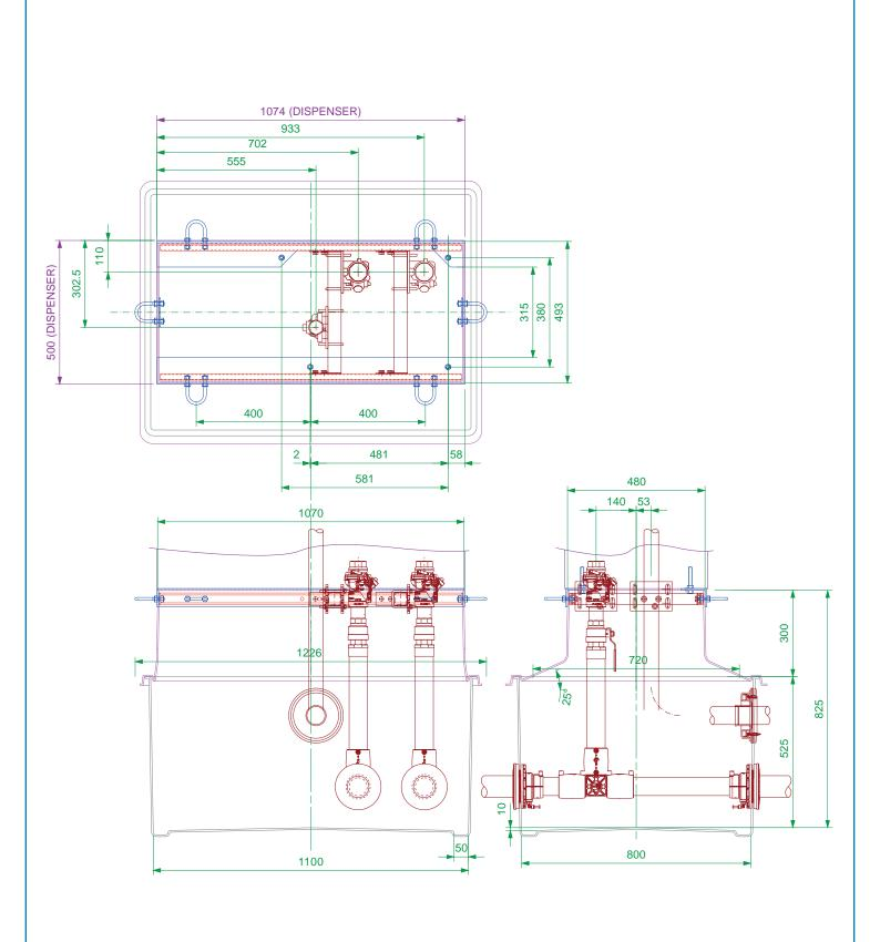
1100mm x 800mm GRP solid base sump and corbel to fit Tokheim Quantium Q510 dispenser model. Includes metalwork. KPS pipework.
