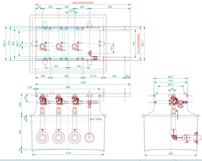
1100mm x 800mm GRP solid base sump and corbel to fit Gilbarco SK700 1/2 dispenser model. Includes dispenser support rails, shear valve rail and all fixings. KPS pipework and Fibrelite entry boots.
