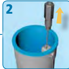
Lift float with cable to simulate fill
